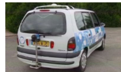
The LARA vehicle from Ecole des Mines, with its laser telemeter
