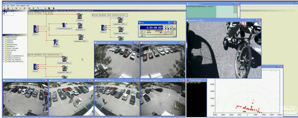
Figure 9 - The PUVAME playback diagram - synchronized playback of 6 infrastructure cameras and on-board sensors
