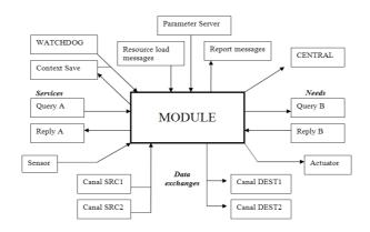
FIG. 2 – Interfaces of a generic module.
