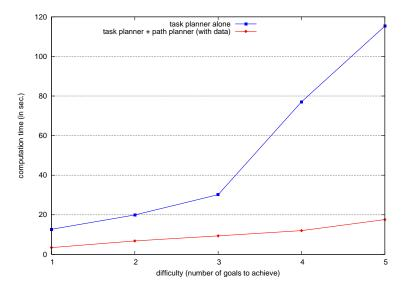
Figure 3: Comparison of the computation time for the two approaches
