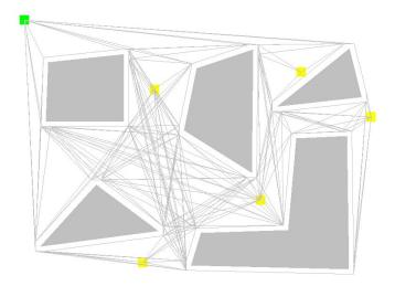
Figure 2: The environment map used with the rover domain and the associated visibility graph
