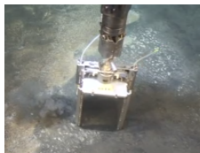
Seabed core sampling
