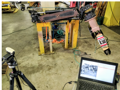
The setup used to acquire the data required for the optimization of the actuators' parameters
