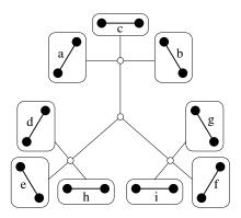
We start with a node containing every edges of the graph, and we *recursively decompose* it until we obtain a *partitioning tree* of the graph.
