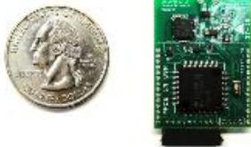
(a) Moo with antenna removed.
