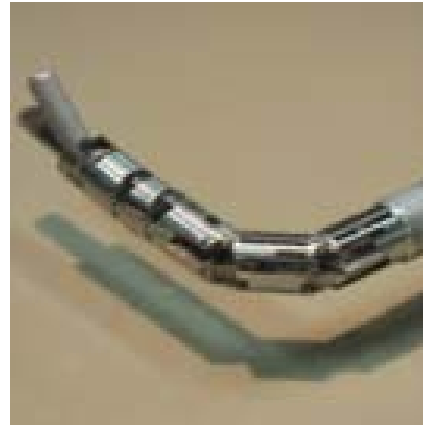
Bending forceps based on rigid linkage mechanism (Univ. Tokyo), 2003
