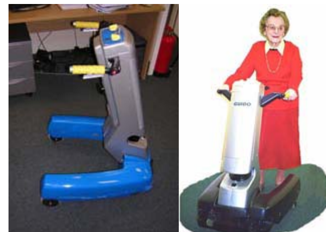
Physical weight support, steered by the user, with assistance to avoid obstacles
