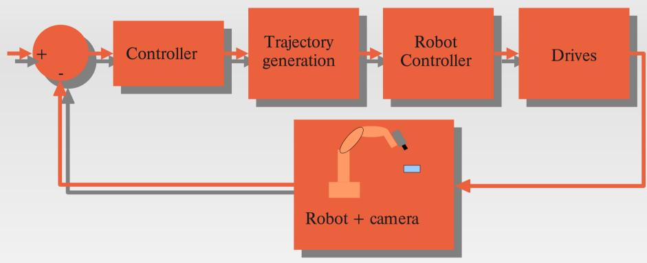
*Indirect visual servoing*: robot joint positions are controlled by the controller provided by the robot manufacturer. The vision loop controller provides velocity control signals which are converted in position setpoints by the robot controller. This type of visual servoing is used when the sampling period is slow thus corresponding to a slow response time.
