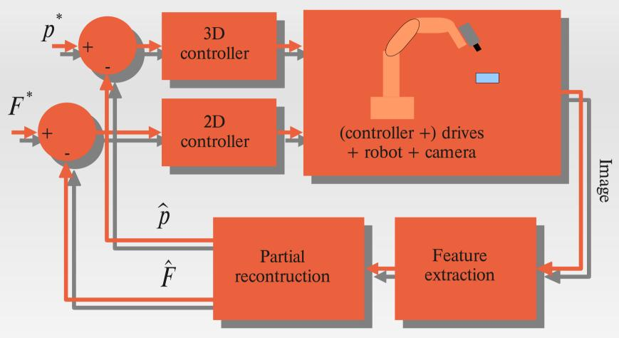
Hybrid (2,5D) visual servoing: some DoFs are controlled in the 3D space and other are controlled in the image plane. The goal is to obtain the best decoupling between the 2 loops.
