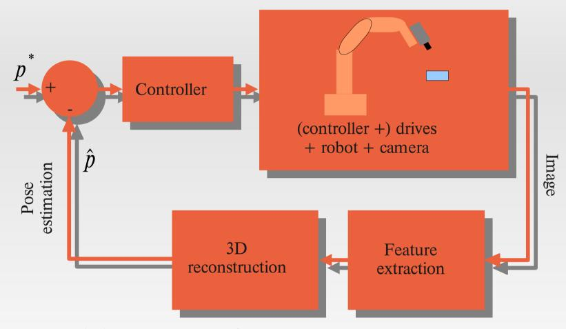
Position based (3D) visual servoing: reference and measurement are poses. To reconstruct the measurement it is necessary to have a model of the object of interest.
