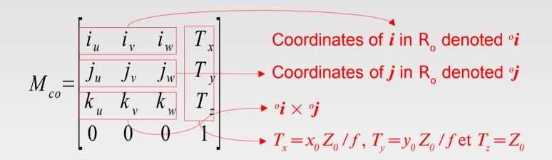
To estimate  $M_{co}$ , it is sufficient to estimate the coordinates of  ${\it i}$  and  ${\it j}$  in  $R_{\rm o}$  and the coordinates of  $M_{\rm o}$  in  $R_{\rm c}$ . The coordinates of  $M_{\rm o}$  in  $R_{\rm c}$ , is obtained from the depth  $Z_{\rm o}$ : if  $x_{\rm o}$  and  $y_{\rm o}$  are the coordinates of  $m_{\rm o}$  in  $R_{\rm c}$  then  $T_{\rm x} = x_{\rm o} Z_{\rm o} / f$  and  $T_{\rm y} = y_{\rm o} Z_{\rm o} / f$
