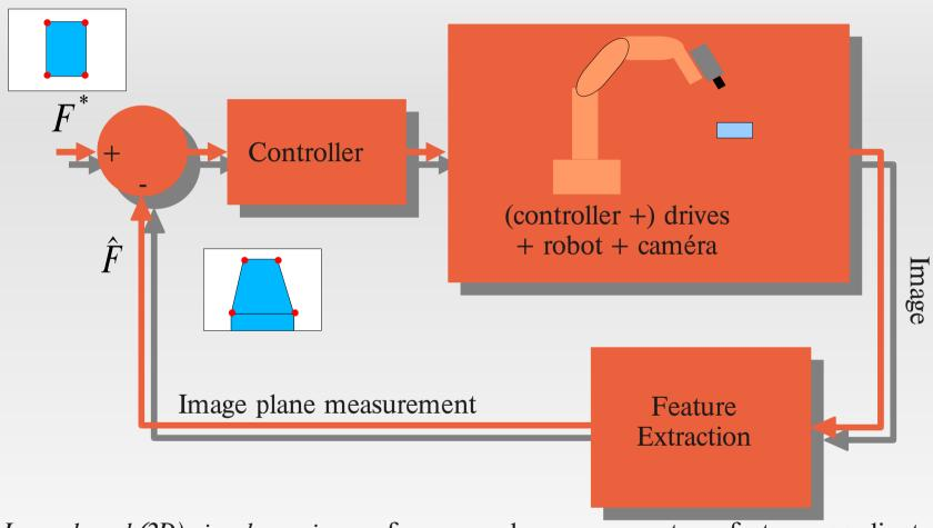
Image based (2D) visual servoing: reference and measurement are feature coordinates. No 3D reconstruction. Not necessary to have a model of the object of interest.
