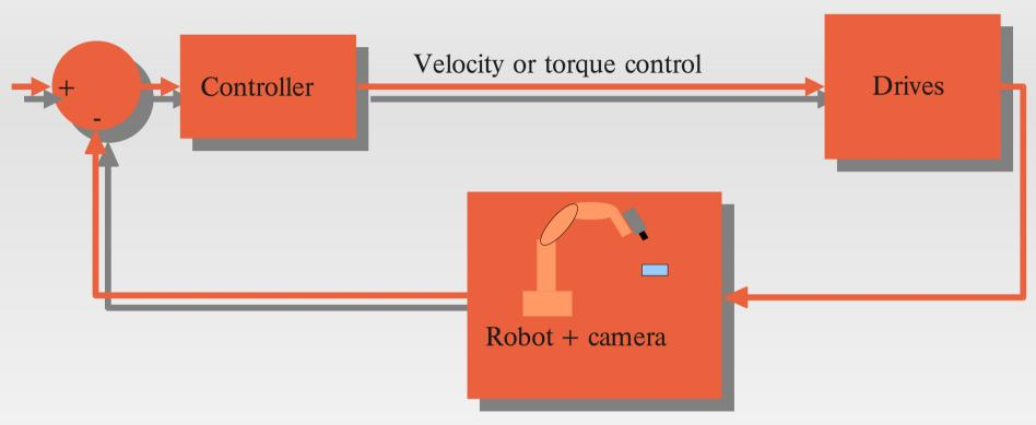
*Direct visual servoing*: robot joints torques or velocities are controlled. Torque or velocity control signals are issued by the controller of the visual loop. They are sent directly to the drives. This architecture is used for high bandwidth visual servoing with a high sampling rate.
