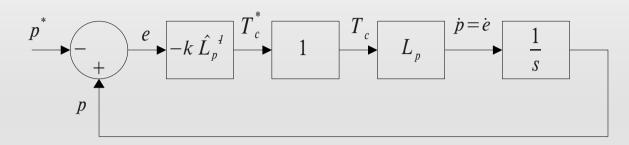
$p^*$ : desired pose p: reconstructed current pose
