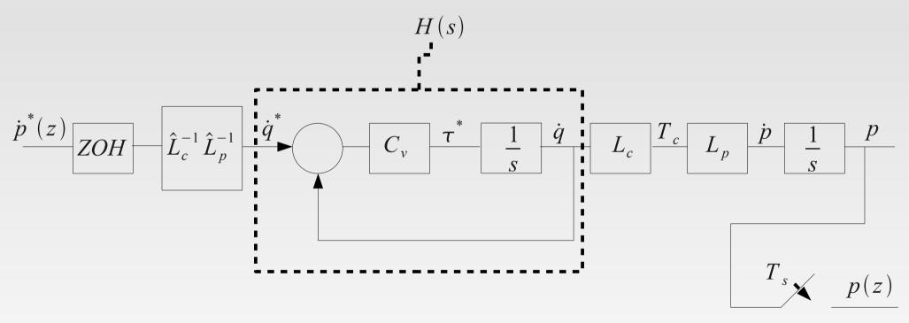
$$T(z) = \frac{p(z)}{\dot{p}^{*}(z)} = (1 - z^{-1}) Z \left\{ \frac{L_{p} L_{c} H(s) \hat{L}_{c}^{-1} \hat{L}_{p}^{-1}}{s^{2}} \right\} \approx (1 - z^{-1}) Z \left\{ \frac{H(s)}{s^{2}} \right\}$$
