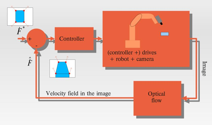
d2D/dt visual servoing: the reference and the measurement are velocities in the image.
