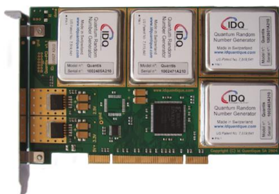
Figure 7 Carte Quantis QRNG PCIe 16Mb
