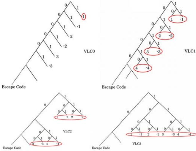
Fig. 3: Tree representation of first four VLC tables used in CABAC. In each VLC table, VLC codes for encircled coefficients have same code length.
