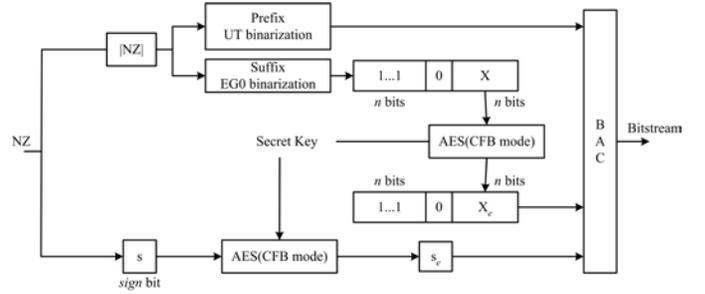
Fig. 9: Encryption process for NZs and their signs in CABAC of H.264/AVC.
