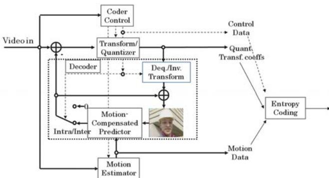
Fig. 1: Block diagram of H.264/AVC video encoder.
