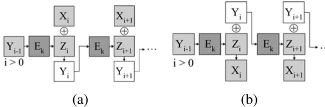
Fig. 5: CFB stream cipher: (a) Encryption, (b) Decryption.
