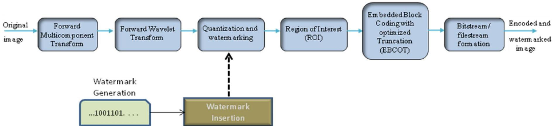
The joint JPEG2000 encoder/watermark embedding scheme.
