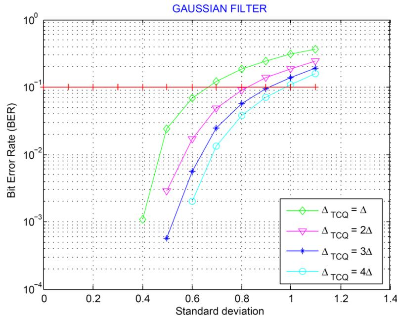
Gaussian filtering attack
