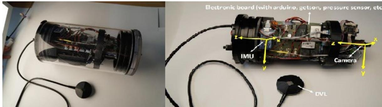
The waterproof underwater capsule of the smart camera system (left) and the smart camera system description with reference frames fixed to it (right)
