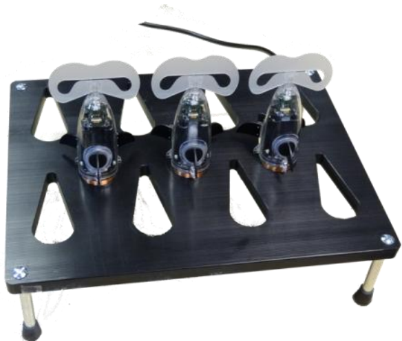
Charging base for 11 robots at slow charging rate (11h)
