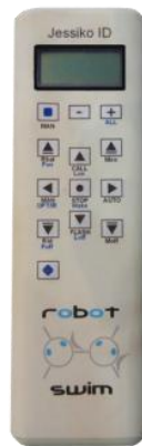
Optical Remote with LCD screen for control and data return from robots
