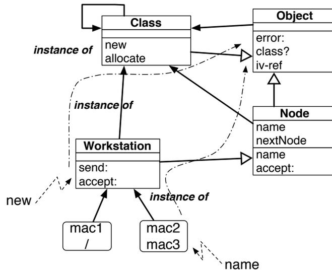
**Figure 1-14** Kernel with instantiation and inheritance link.
