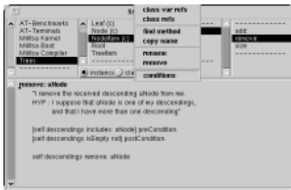
Figure 4 : The currently selected class ( NodeItem ) has its conditions activeness set (cf (c)). The associated conditions codes is executed at runtime. The figure also shows the menu (conditions) that permits the change from active to non-active conditions (and vice versa).
