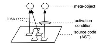
**Figure 1** Metalinks installed on the AST
