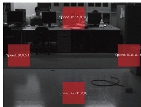
Fig. 3. Static interface with speed (forward, sideways, rotation) in m/s associated to the stimuli (capture of a video streaming feedback from the embedded robot camera).
