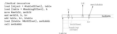
The method table consists of the hashtable, which contains a single entry per method or class. With dynamic typing, the method identifier (methID) must be checked in the method prologue, unless the method has been introduced by the hierarchy root.
