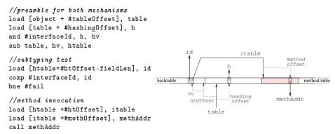
The method table is bidirectional. Positive offsets contain method addresses and class IDs, as in SST, and negative offsets consist of the hastable, with a twofold entry for each implemented interface. The grey rectangle denotes the group of methods introduced by the considered interface. fieldLen represents the entry size, e.g. 8 if 32-bit integers are used. In practice, all numbers (i.e. H and class ID's) must be multiplied by fieldLen (of course, it works only if it is a power of 2).
