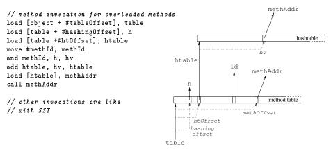
The method table is the same as with SST, apart from two extra fields for referencing the hashtable (#htOffset) and the hashing parameter (#hashingOffset), which can be loaded in parallel on processors that provide instruction-level parallelism. The hastable contains a single entry per method, only for methods that have been introduced by more than one class.
