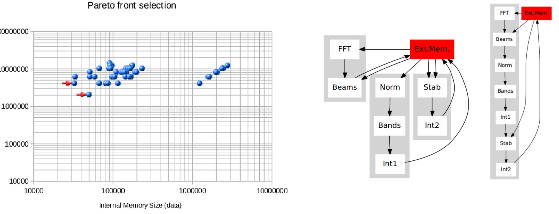
The design space contains 54 fusions and 2 are selected. The exploration lasts 3 seconds.
