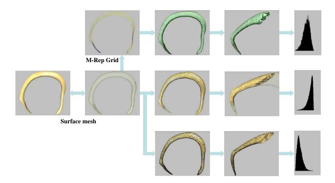
Fig.1. Comparison between tetrahedral meshes generated by the three techniques. From top to bottom: VMBM-rep, VTM and TetGen. From second to fourth column: Whole volumetric mesh, detail of a thin part, aspect ratio histogram.
