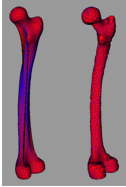
Figure 4.6: Left: The non-optimised femur model presents a poor topological and geometrical quality. Right: desired model with quasi-regular faces
