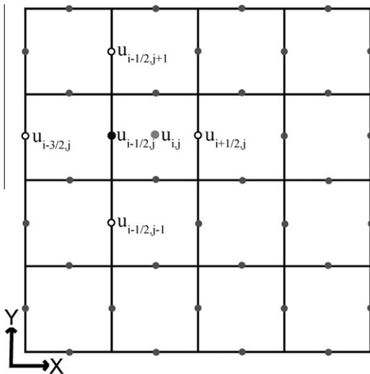
Fig. 1. A diagram of the nodes used to compute the Laplacian at node  $u_{i-1/2,j}$  which is depicted by the solid black circle. Neighboring nodes are shown as hollow circles.
