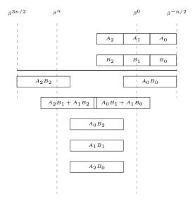
Figure 2: Reducing the number of call to **PMR** and **PBR** in the 3-ary multipartite algorithm by accumulating partial products of identical weight
