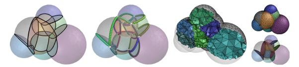
Figure 2.3: (Left) A set of curves are extracted where three or more labeled regions intersect. (Middle) these curves are protected with an initial set of balls that may get refined by the algorithm later. (Right) resulting mesh generated by converting these balls to weighted points and refinement fills in samples for the interface surfaces [DJL12].
