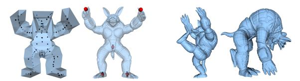
Figure 3.5: Deformations of the Armadillo model using variational harmonic maps [BCWG09]. (Left) Cage and anchor locations along with the original pose and constraints. (Right) Deformed poses.
