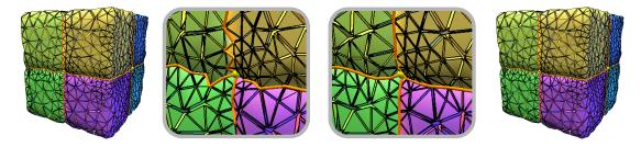
Figure 2.21: **Feature preserving smoothing.** Using the feature complex, a feature preserving hierarchical smoothing is performed.
