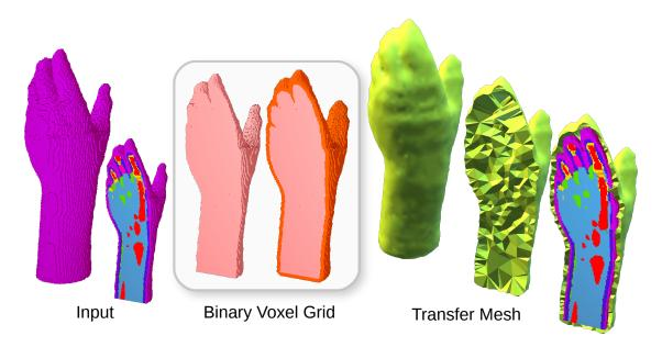
Figure 3.15: **Transfer mesh**: an adaptive Delaunay tetrahedral mesh undergoes the ARAP/GC deformation defined interactively and transmits it linearly to the input voxel grid for a limited per-voxel computational cost.
