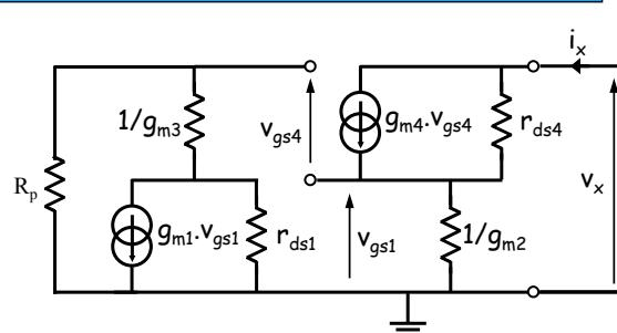
$$i(R_p) = \frac{r_{ds1}}{R_p + r_{ds1} + \frac{1}{g_{m3}}} g_{m1} v_{gs1}$$
