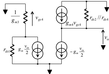
$$v_{out} = \left( g_{m4} v_{gs4} + g_m \frac{v_{in}}{2} \right) \times (r_{ds2} // r_{ds4})$$
