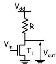
$$V_{in} = V_{dc} + v_{in} \cong V_{eff} + V_{in}$$
