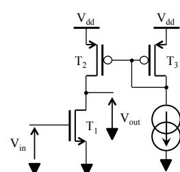
$$A_V = -g_{m1} \left( r_{ds1} // r_{ds2} \right) = \frac{-g_{m1}}{(g_{ds1} + g_{ds2})}$$
