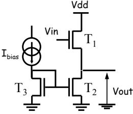
$$V_{gs1} = V_{in} - V_{out}$$
