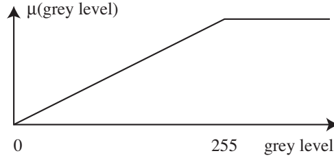
Figure 20: Mapping membership functions to grey levels
