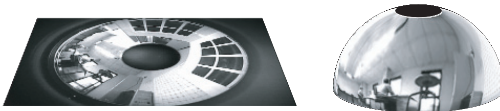
Figure 9: Projection of the Daniilidis dome.
