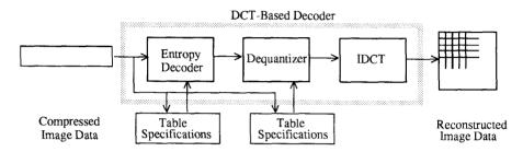
Figure 2. DCT-Based Decoder Processing Steps
