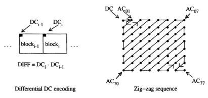
Figure 3. Preparation of Quantized Coefficients for Entropy Coding
