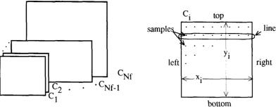
(a) Source image with multiple components (b) Characteristics of an image component
