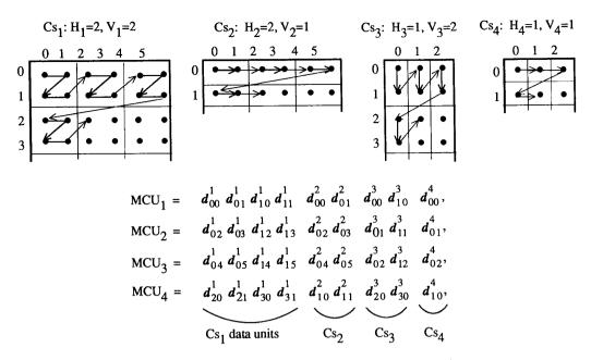
Figure 8. Generalized Interleaved Data Ordering Example
