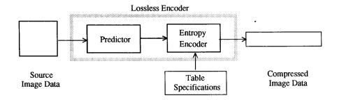
Figure 4. Lossless Mode Encoder Processing Steps
