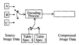
Figure 9. Component-Interleave and Table-Switching Control
