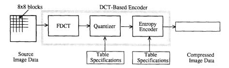
Figure 1. DCT-Based Encoder Processing Steps
